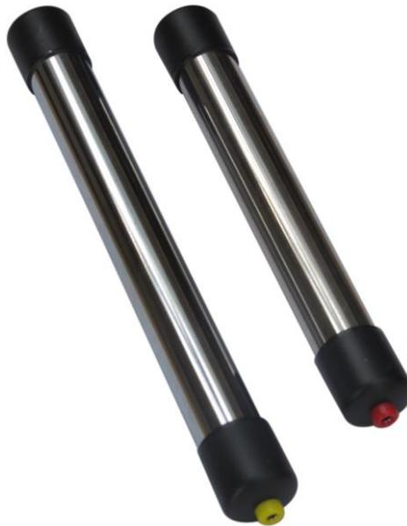
The hand probes are connected with the corresponding colored banana plug cables. Keeps red to red and yellow to yellow, put one end of the cable into the MTD unit and the other end of the cable in hand probe.
